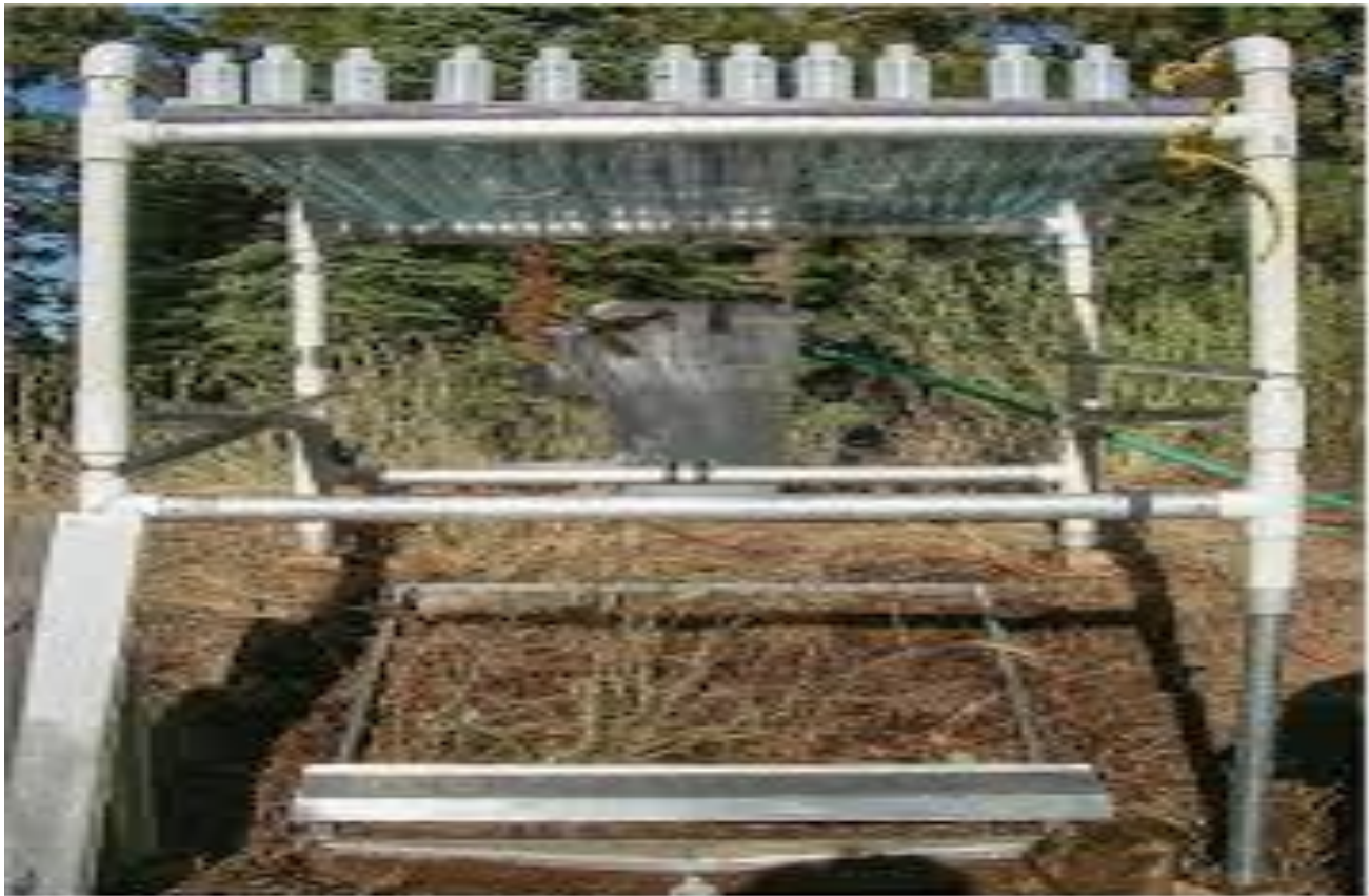
This simulator uses a frame with nozzles (top) to apply water at various rates and a frame on the ground to catch sediments.
